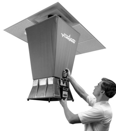
This meter can be installed on the **FlowHood** in less than 60 seconds. Air flow readings are automatically corrected for air density and backpressure at supply or exhaust outlets.
